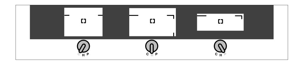
The view through the finder will change to the style of photographs shown when the print format switch is operated. The angle of the exposure will not change.
